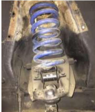
*Figure 3 Before removing factory spring.*
