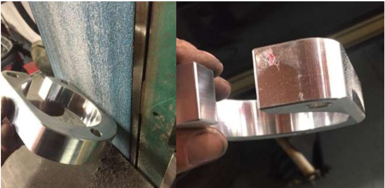
*Figure 8 Showing modification and after modification of shock spacer.*
