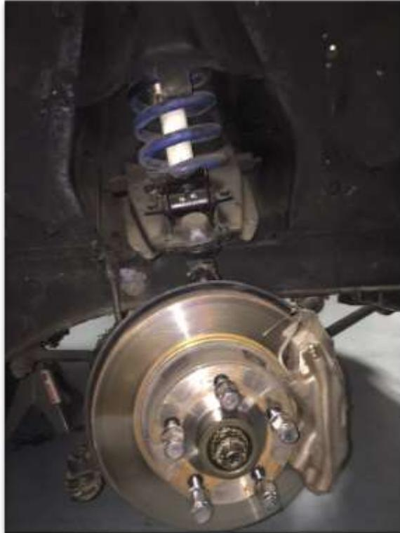
3. Disconnect the front sway bar end link from the lower control arm on both driver & passenger sides.
