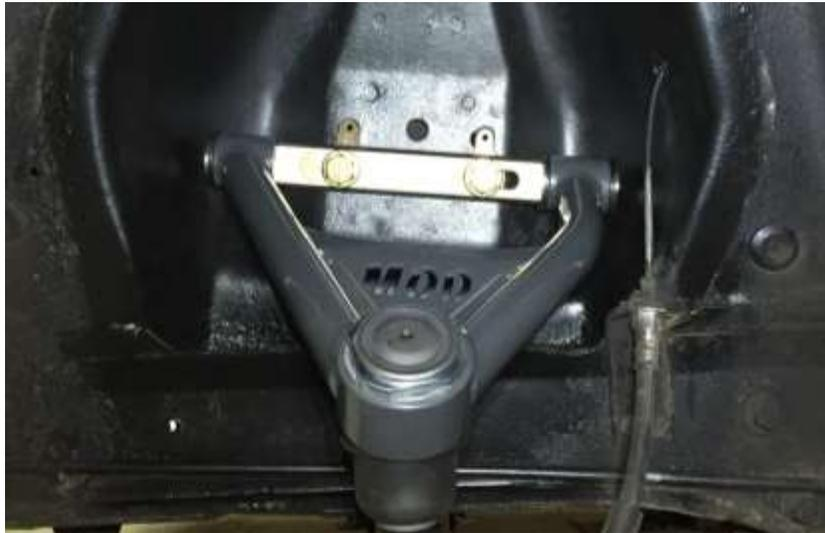
Figure 10 Upper control arm installed in vehicle. Note: Front of vehicle is on left side of the page
