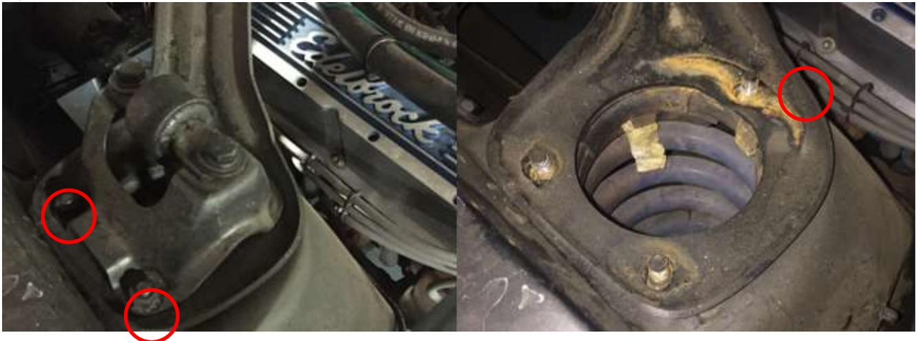
Figure 2 Shock & Shock Cap Removal.
