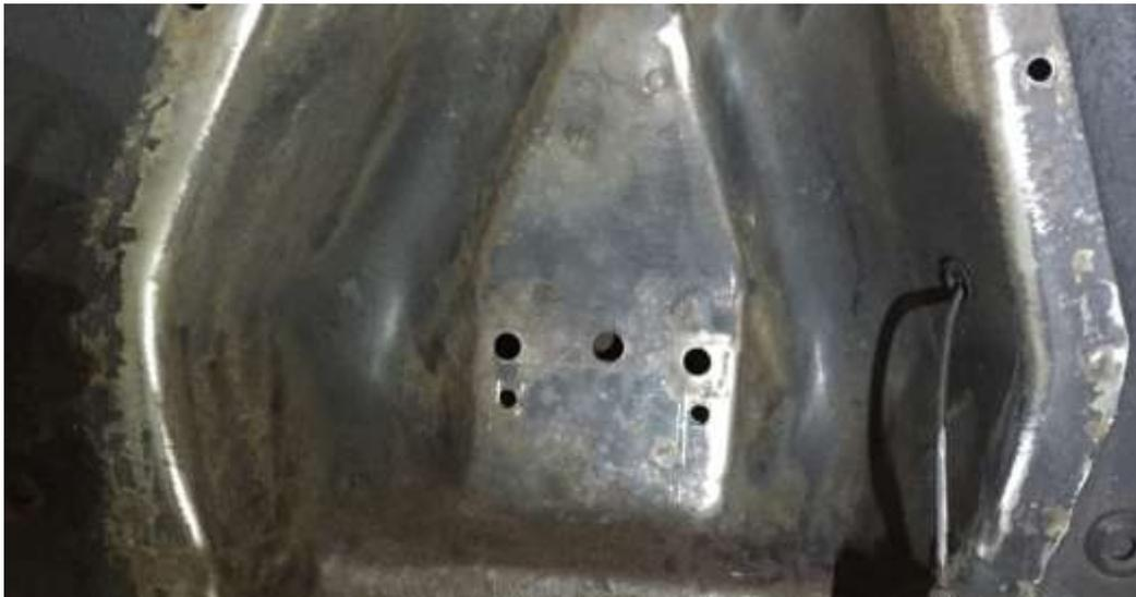
*Figure 6 Shock tower wire wheeled and pilot holes drilled for Shelby drop on a 1964.5-1966 Mustang*
