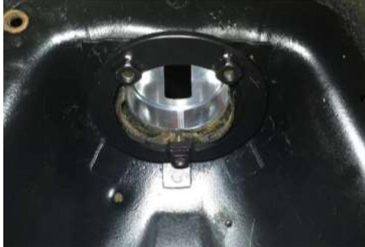
Figure 9 Shock top assembly installed
