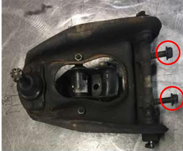
*Figure 5 Upper control arm removed from vehicle showing hardware to be removed from UCA.*
