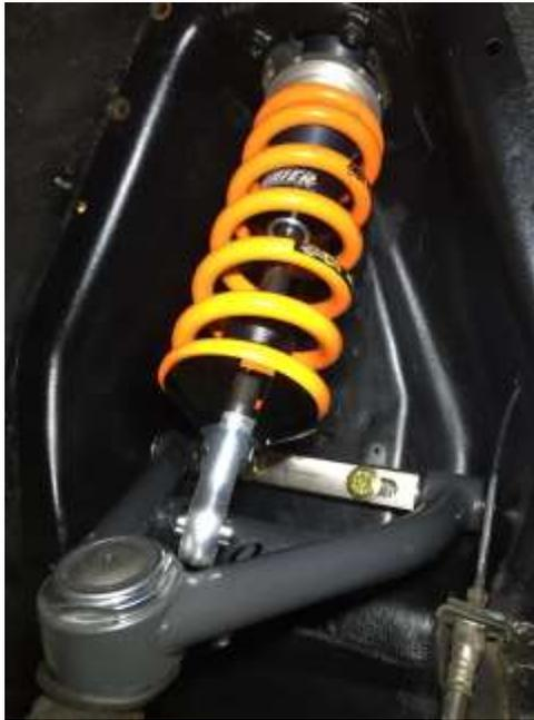
Figure 11 Coilover shock partially installed.
